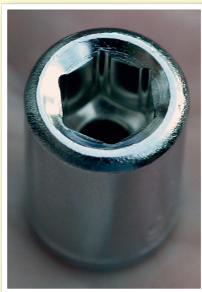
One of the easiest ways of spotting dubious quality is excessively fat socket walls, like here.
